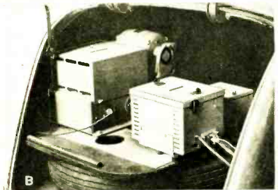
Upper-Left: New 25-watt police radio xmtr, as set up on a Despatcher's desk in headquarters. Lower Left: The 15-watt crystal-control UHF receiver & dynamotor, mounted in the rear trunk of a 1938 Ford. The receiver is in the foreground. Above: Control unit & handset mounted on dash of same car. All equip't in this layout is G-E except handset, which is by Automatic Electric Co.
